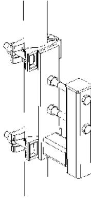
Figure 49. Scaffold attachment installed on a standard
