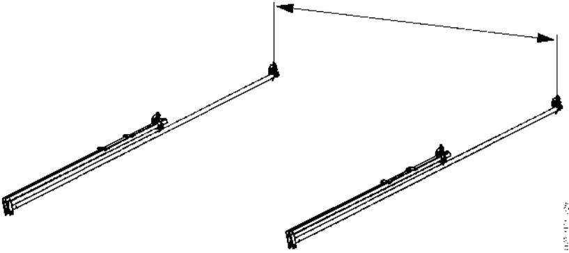
*Figure 27. Place the frames with the correct c-c spacing*
