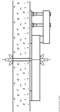
Figure 45. Facade attachment installed through a wall
