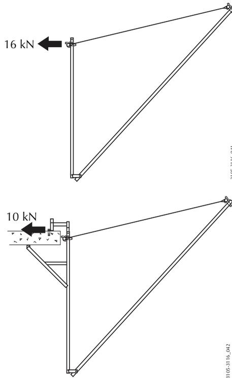
Figure 40. Anchorage loads
