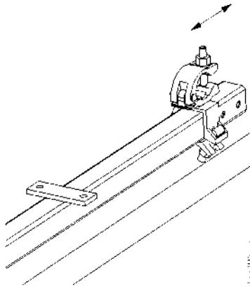
Figure 26. Positioning of square-round coupler
