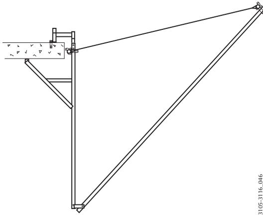
Figure 44. Safety net fan lifted into position
