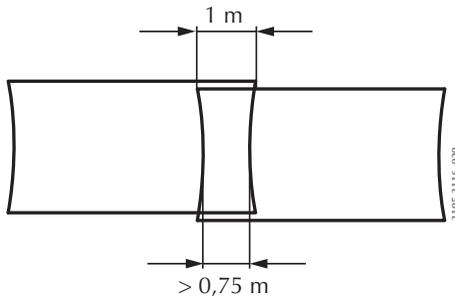
Figure 17. Fall-arrest fan overlap
