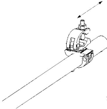
Figure 24. Adjust the double coupler spacing
