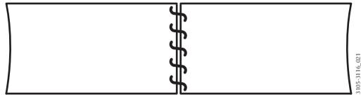
*Figure 18. Joining nets by lacing*
