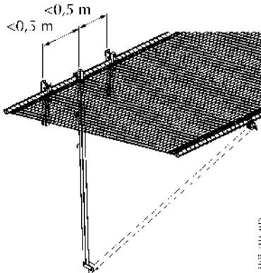
Figure 46. Positioning of the facade attachment
