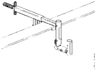
*Figure 53. Multi-clamp with elbows installed on a wall top/upstand*
