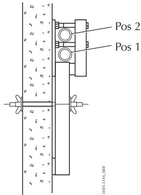
Figure 47. Levels within the facade attachment
