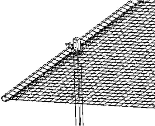
Figure 35. Thread the frame through the net.
