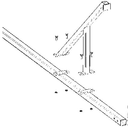
*Figure 41. Assembling the knee brace on the frame*
