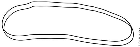
*Figure 12. Lifting sling*
