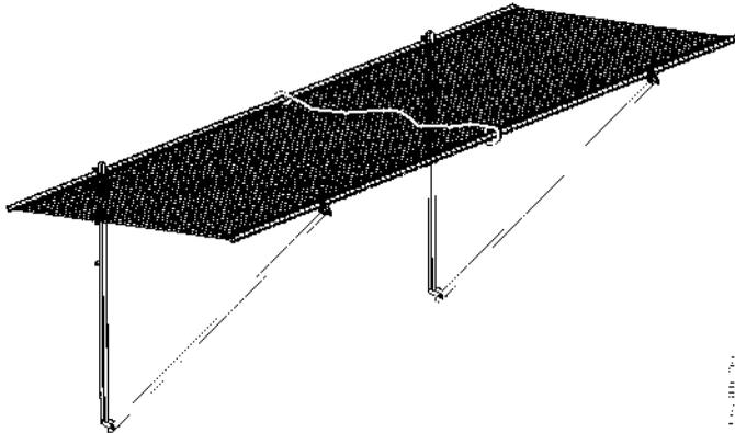
Figure 38. Assembled safety net fan
