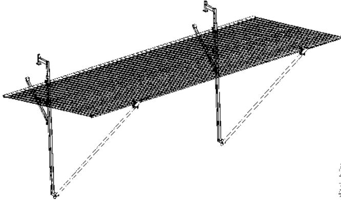
Figure 43. Safety net fan ready for installation on the slab
