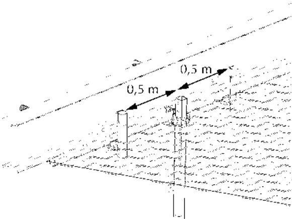
*Figure 58. Positioning the steel jaw clamps*
