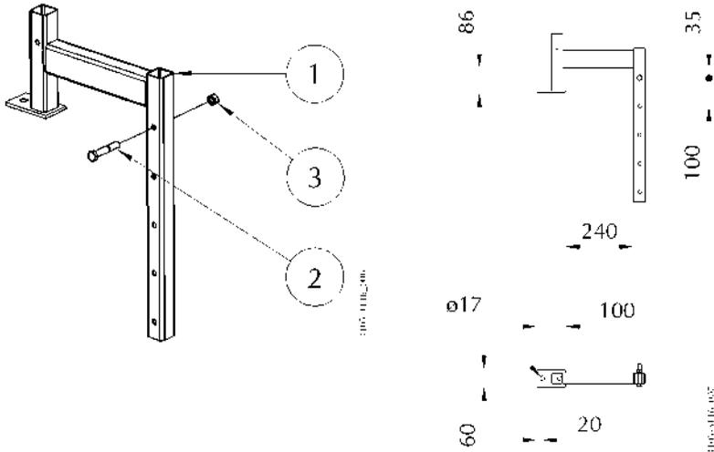
Figure 7. Slab attachment
