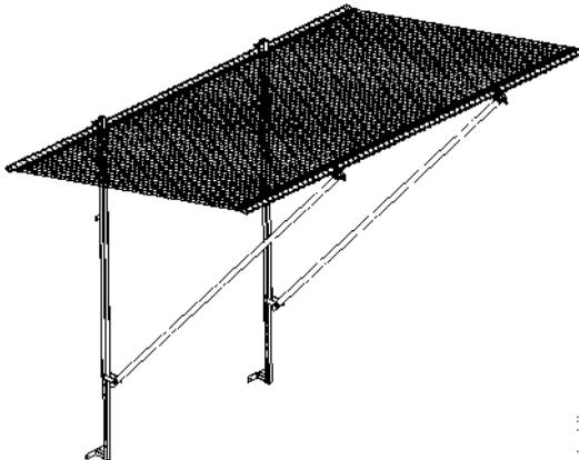
Figure 62. Safety net fan with extension
