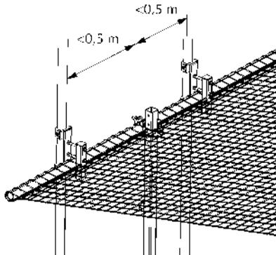
Figure 50. Positioning the scaffold attachment
