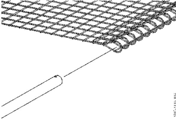
*Figure 31. Threading the tubes to the fall-arrest fan net*
