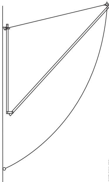
Figure 20. Tying down the safety net fan for high wind
