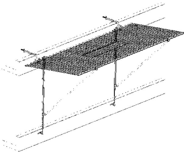
*Figure 56. The safety net fan installed with the multi-clamp*
