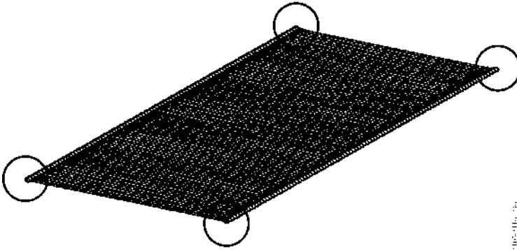
*Figure 33. Secure all four corners of the net*
