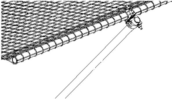
Figure 37. Assemble the outer tube on the raking tube
