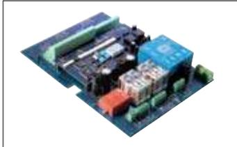
Betafence has developed a high quality steering unit. A control unit with microprocessor manages the general functions and contains the control logic. A separate unit contains the special functions for access control.
