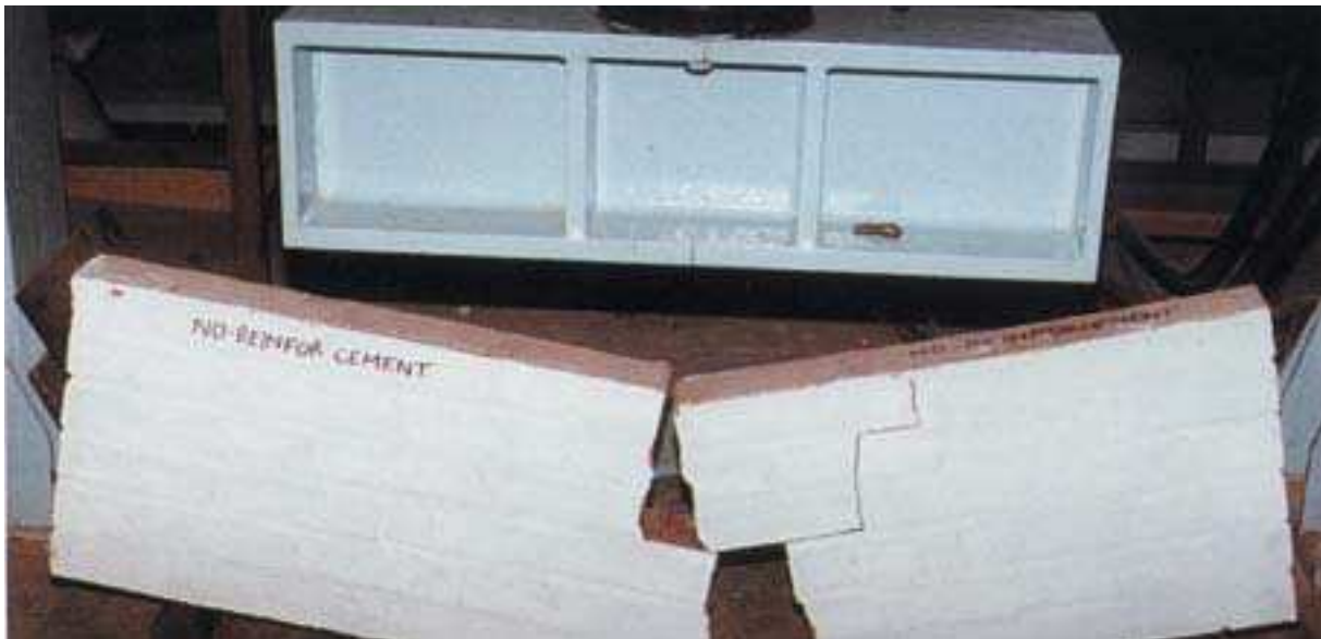
Destruction testing of un-reinforced wall
